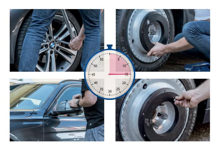
"With our wheel torque transducers, we provide our customers with high-precision tools for measuring the torque at the wheel. We have consistently paid attention to short set-up times and easy, convenient handling during assembly. The synchronous, cable-free acquisition of measurement data is made with standard components of the D<sup>x</sup> telemetry, thus ensuring optimum transmission quality."
