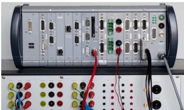
Abb. 3: imc CRONOScompact: universal modular measurement system with HiL extension (embedded simulation processor)
